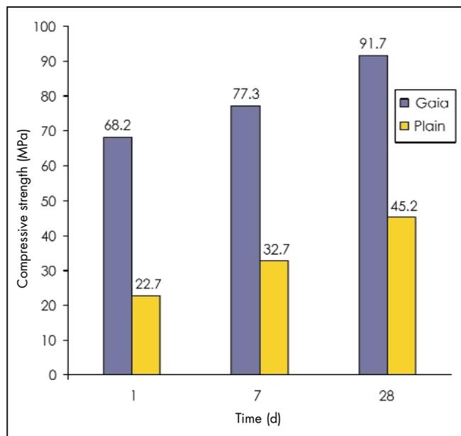
Figure 8 Strength development of concrete with Gaia.
