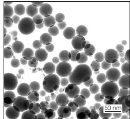
**Figure 7** Ultrafine fumed silica particles observed using TEM.<sup>37</sup> Courtesy Andri Vital, EMPA Mat's Testing & Research, Laboratory for High-Performance Ceramics, Dübendorf, Switzerland.
