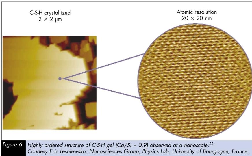
**Figure 6** Highly ordered structure of C-S-H gel (Ca/Si = 0.9) observed at a nanoscale.<sup>33</sup> Courtesy Eric Lesniewska, Nanosciences Group, Physics Lab, University of Bourgogne, France.
