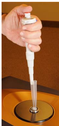
Figure 6 Pipette and silicone tubing attachment to reference cell access tubes.
