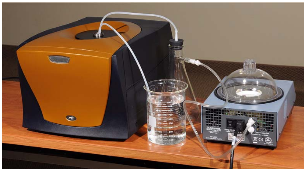
Figure 11 Capillary cell cleaning apparatus for flushing large volumes.
